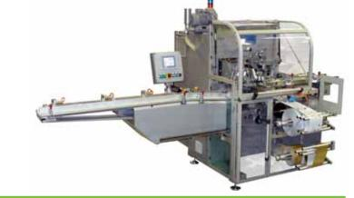
One-step wrapping machine for chocolate bars and tablets in envelope style with single or double wrapping material fed from reel, closed by hot melt glue. The machine is suitable for a wide range of product, from small bars up to large tablets.
