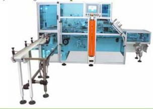
Two-step wrapping machine for chocolate tablets. First step with alufoil sealed on 3 sides; Second step either with paper in envelope style or banderole or carboard closed by hot melt glue.
