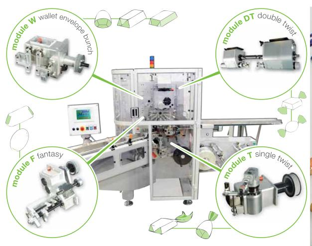
SWEET MAGIC is a MULTYSTYLE wrapper for chocolate pralines. Its peculiar modularity is conceived to complete the basic SM machine with up to 4 different wrapping units, enabling to obtain many different wrapping styles. The machine may be equipped with an automatic aligner and/or vibrating hopper to optimize product feeding.
