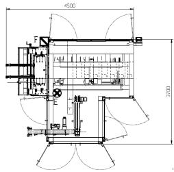
Example of layout for flat base box configuration
