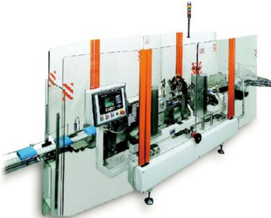
Layout of a typical 1 Flap Box closer (BC1) (mirror version available)
