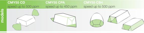
MONOSTYLE belt-feeding wrapping machine for flat-base chocolate pralines. Each version is dedicated to a specific style (Double twist, Bunch/Envelope/Wallet, Open points) and is suitable for all the most common wrapping materials. The machine can be equipped with an automatic aligner to optimize product feeding.
